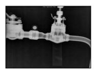
Similar to film radiography with distinct advantages such as digital images, less consumables, lower infrastructure cost, lower radiation, shorter exposure times, no darkroom and less retakes. Particularly useful for CUI and small bore pipework inspections.
