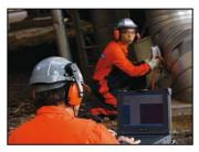
Pulsed Eddy Current (PEC) is an inspection technique that can measure wall thickness of steel objects such as pipes and pressure vessels without making contact with the steel surface, through coatings, insulation materials and even corrosion products.
