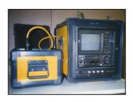
COBRA is a miniature gas safe CCTV system which has been designed for the thorough examination and recording of difficult access areas such as pipework, pressure vessels, ship's bottom plating underneath bellmouths etc.
