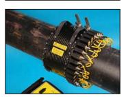
Long range ultrasonic testing is a low frequency ultrasonic technique used to detect defects and imperfections some distance away from the ultrasonic source in a range of components. Particularly used in the detection of corrosion and metal loss in pipes and pipelines.
