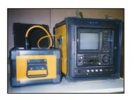
SNOOPY is a method of in-water and subsea visual and ultrasonic surveys for ships and floating and fixed offshore installations which avoids the need for support vessels, tank cleaning etc. Tanks can remain in service throughout the survey.
