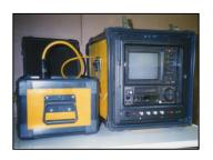
CYCLOPS is a helmet mounted CCTV system. EM&I specialist technicians have the ability to transmit visual and audio survey data to a console, which allows communication between the technician and owner/ operator and/ or the regulator representative.
